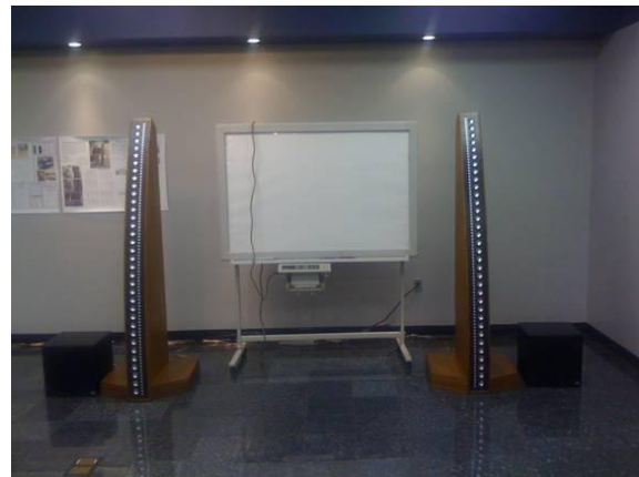
Fig. 1. A pair of prototype CBT30 ground-plane CBT arrays set up in the car lab at Harman's Northridge California campus for stereo listening (note flanking subs). The room is approximately 20 ft wide, 55 ft long, with an 8.5 ft ceiling.
